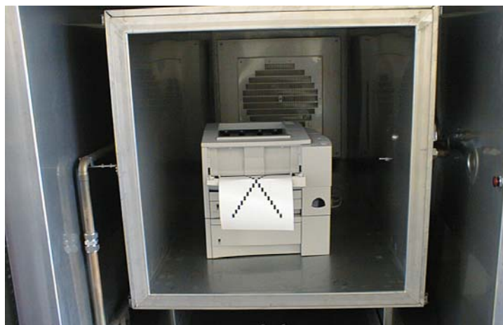
Figure K1: View of the type B 1m 3 emission test chamber with a printer in test
