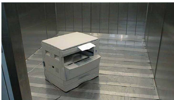
Figure K2: View of the 20m 3 emission test chamber with a printer in test
