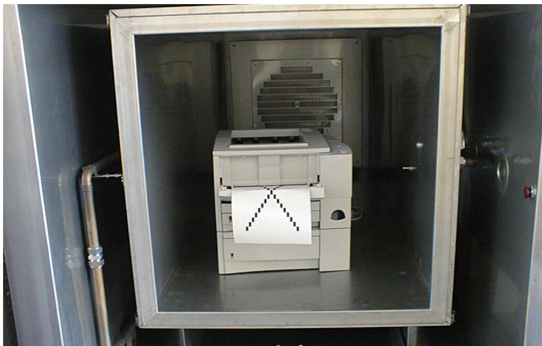
Figure 1: View of the 1-m<sup>3</sup> emission test chamber loaded with a printer
