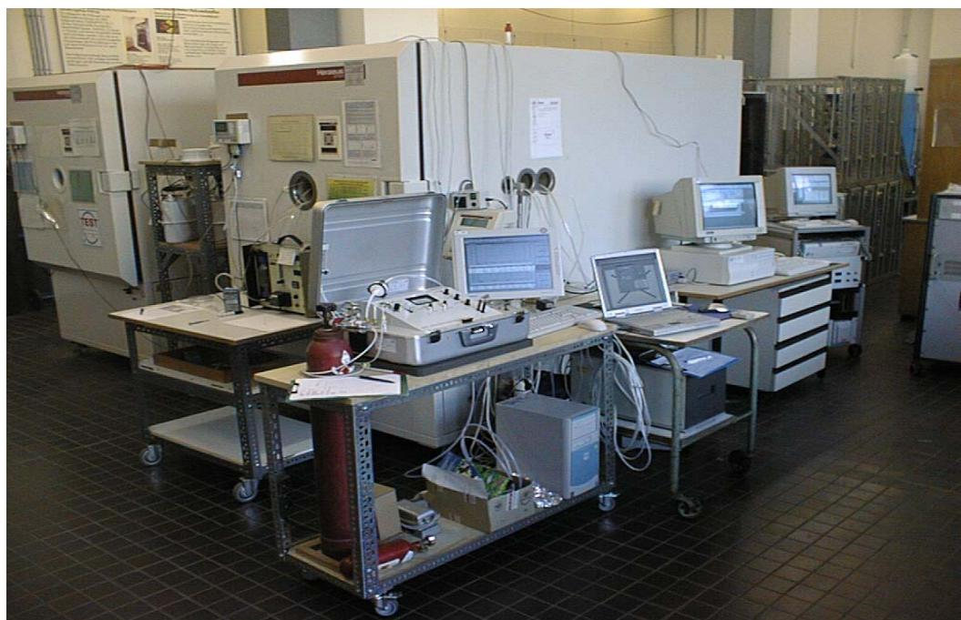
Figure 2: 1-m<sup>3</sup> emission test chamber, complete measuring station
