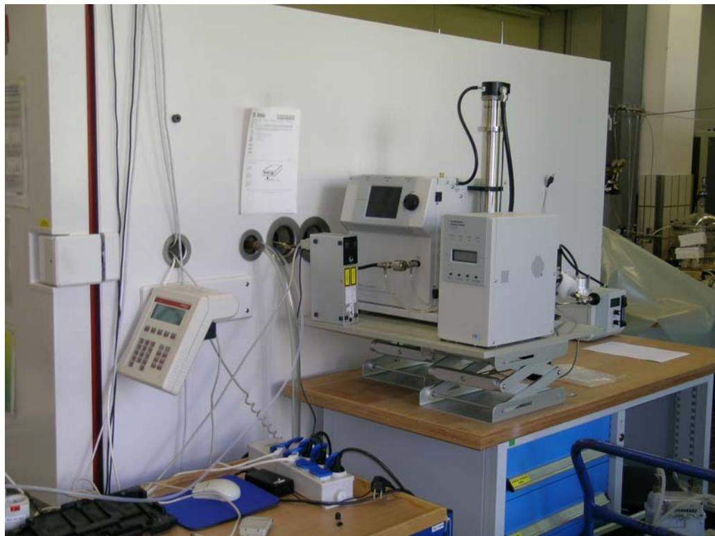
Figure 59: Arrangement of the particle spectrometers at the 1 m<sup>3</sup> test chamber
