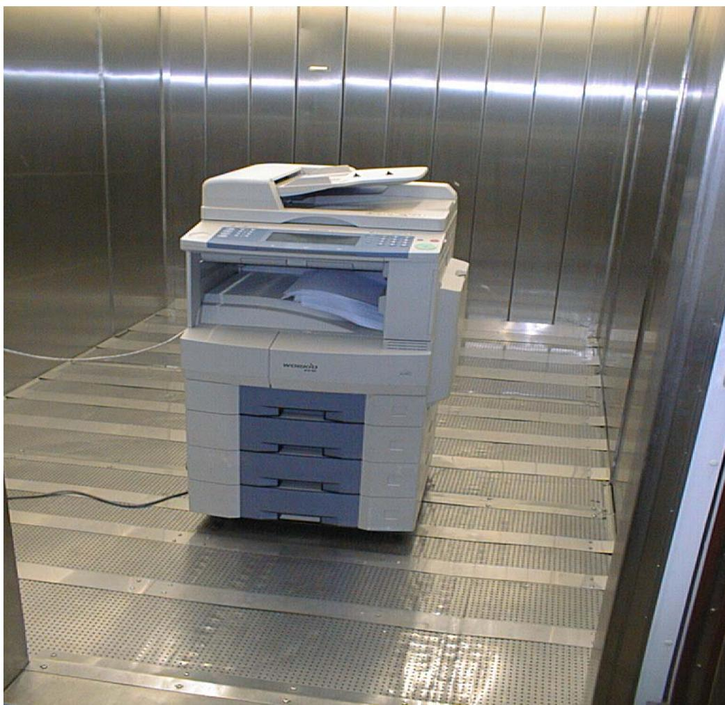
Figure 3: 20-m<sup>3</sup> emission test chamber with a printer
