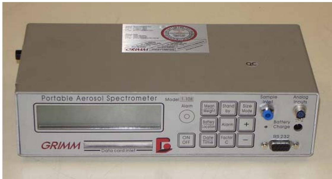
Figure 57: Particle spectrometer Grimm 1.108 Portable Aerosol Spectrometer
