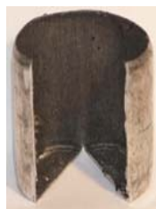
Fig. 4: Mechanical pretreatment of dry cells (zinc/carbon)
