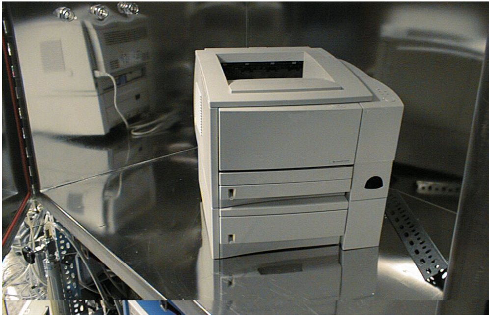
Figure 9: View of the type A 1m 3 emission test chamber with a printer on test
