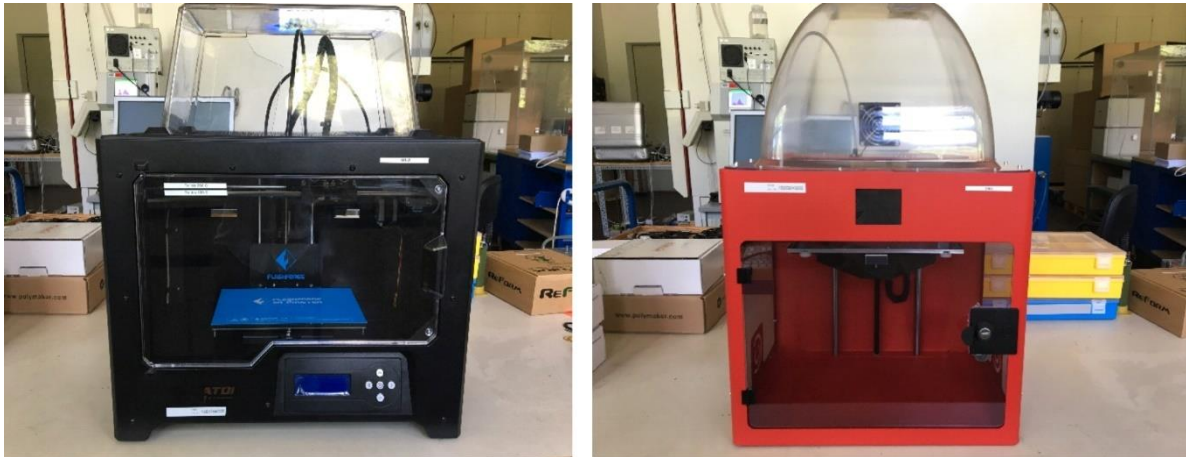
Frontansicht der FFF-Drucker, links: FFF1 (Flashforge Creator Pro™), rechts: FFF2 (Craft Bot 2™); © BAM.
