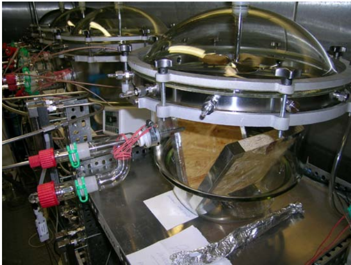
Figure 2: 23-litre emission test chamber
