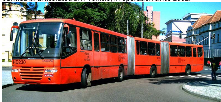
Curitiba bi-articulated BRT vehicle, in operation since 1992.
