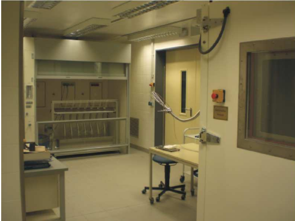
Figure 4-28: Mobile comparative scale and 5-m 3 chamber with assessment funnels
