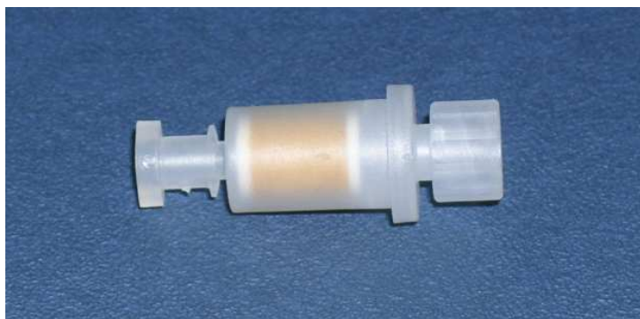
Figure 4-23: DNPH sampling cartridge for aldehydes and ketones
