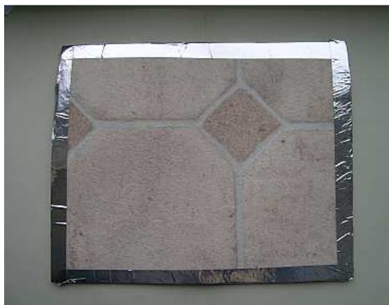
Figure 4-14: Two PVC samples prepared for the 24-litre chambers
