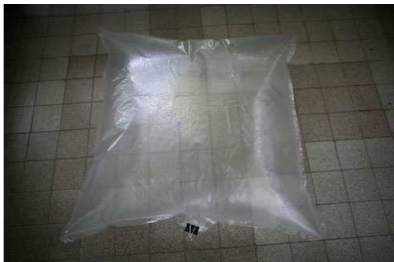
Figure 4-11: Tedlar® container filled with sample air
