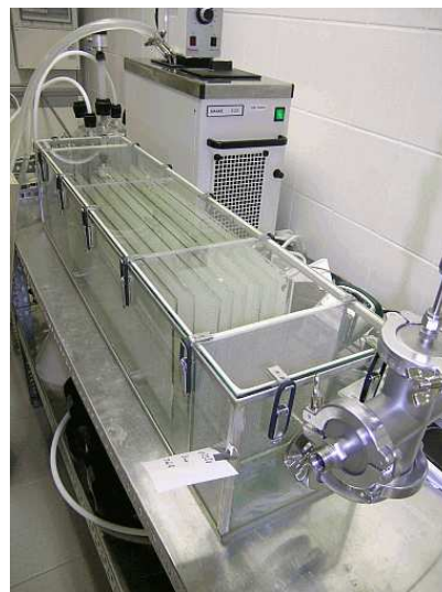
Figure 4-5: CLIMPAQ (44-litre chamber)
