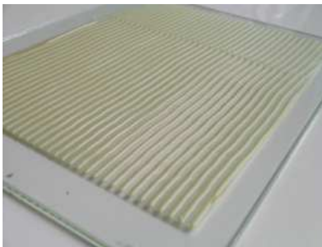
Figure 4-15: Application of a floor covering adhesive on a glass plate
