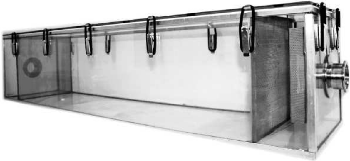
Figure 4-7: Photograph of a CLIMPAQ used at HRI
