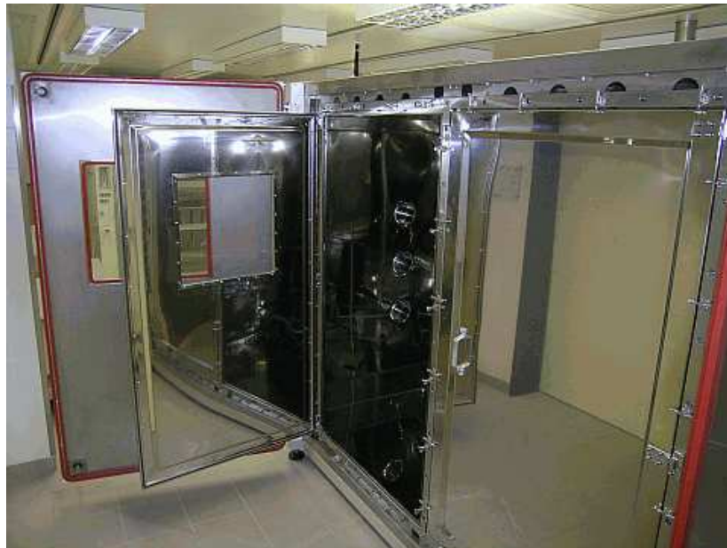
Figure 4-8: 5-m 3 chamber with the door open
