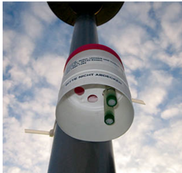
Passive collector: A passive collector is a small monitoring device which operates without electrical power and in which several detection tubes absorb the pollutants from the air. The detection tubes are regularly removed and their contents evaluated in the laboratory.
