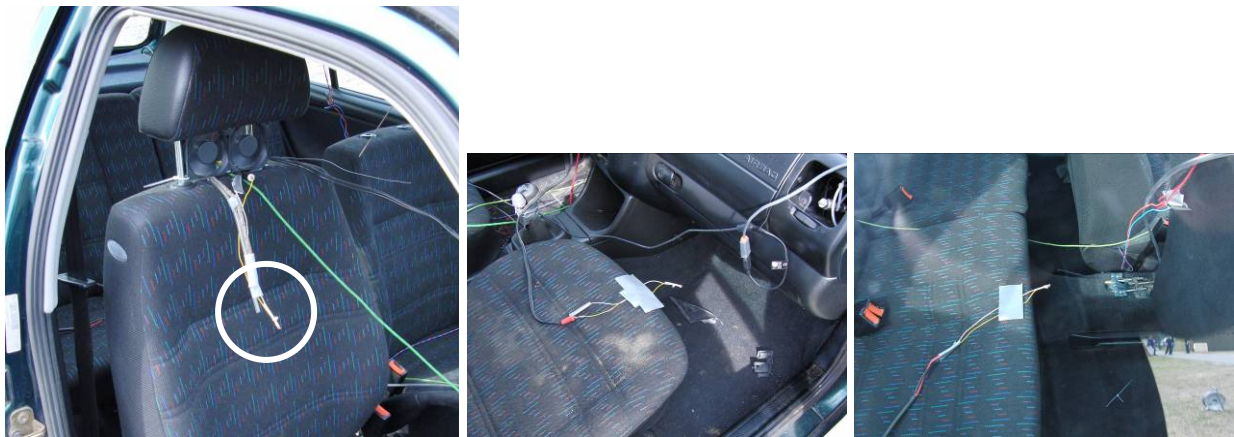
Fig. 22: Location of the modified pyrotechnical igniters for match ignition and location of the O 2 -analysis tube
