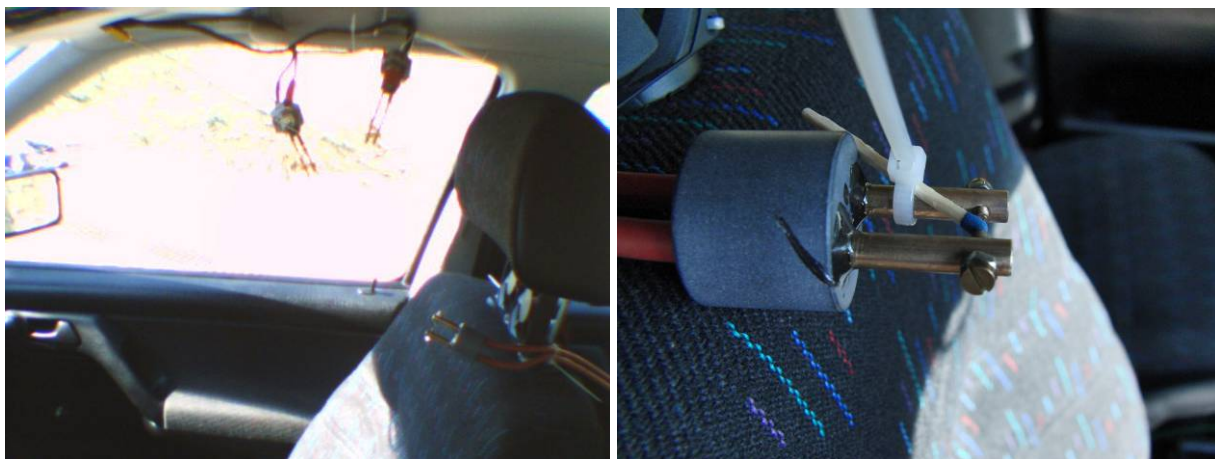
Fig. 19: Location of ignition sources in order to ignite a leakage stream of HFO1234yf (left picture: high voltage spark and “exploding wire”; right picture: modified high voltage spark for the ignition of a match)
