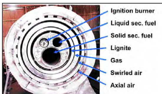
Figure 2.14: Front view of a multi-channel burner used in a rotary kiln (RK)
