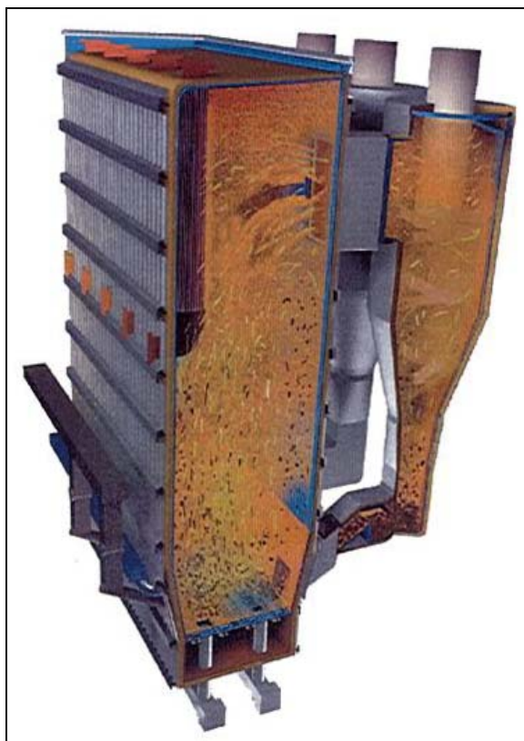
Figure 5.7: Fuel and bed material flow in a biomass fired CFBC boiler [91, Kokk, et al., 2000]
