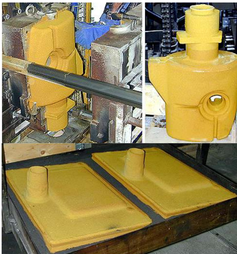
Figure 2.33: Curing cores (top) and moulds (bottom) [237, HUT, 2003]
