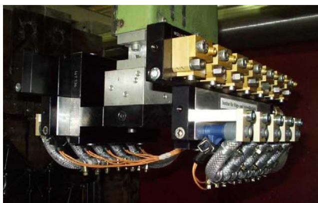
Figure 6.1: Spray head with separate nozzles for water and release agent
