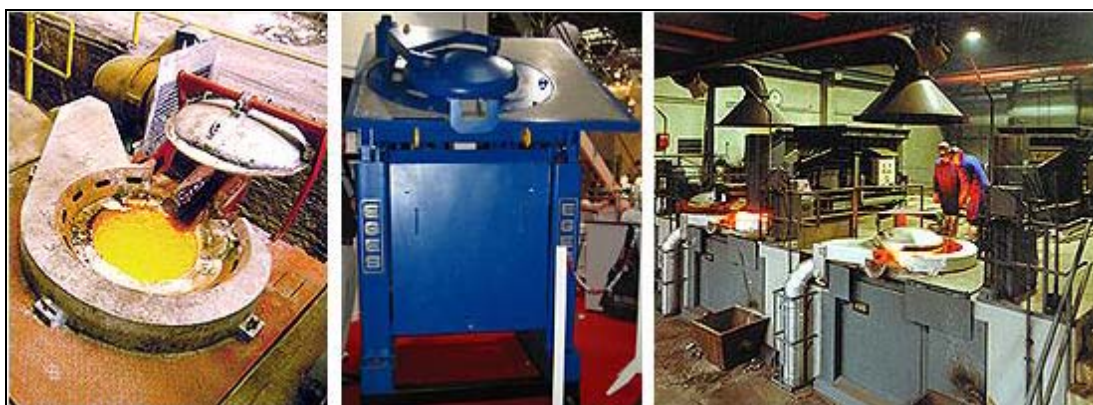
Figure 2.14: Coreless induction furnaces [237, HUT, 2003]
