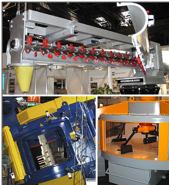
Figure 2.29: Various types of sand mixers [237, HUT, 2003]
