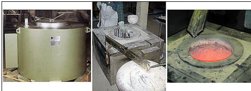
Figure 2.20: Crucible furnaces [237, HUT, 2003]
