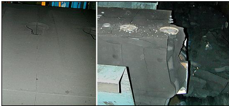
Figure 2.43: Shake-out at the end of an automated moulding line [237, HUT, 2003]
