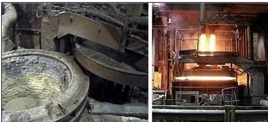
Figure 2.12: EAF furnace [237, HUT, 2003]
