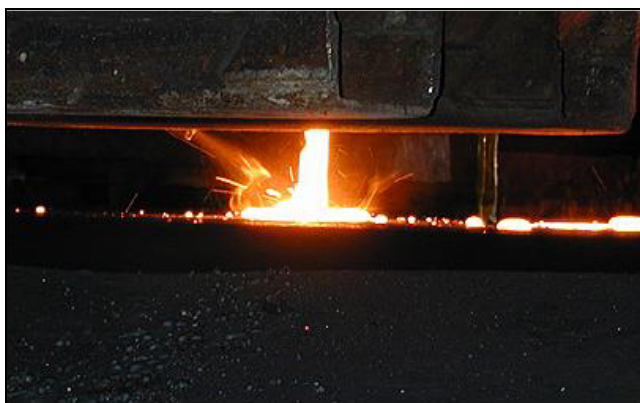
Figure 2.24: Inoculation during pouring [237, HUT, 2003]
