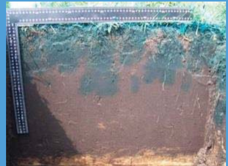
Top: Cracks in clay soil (Credit: with kind permission from Bram te Brake). Bottom: Preferential flow patterns through soil (Credit: with kind permission from Esther Bloem)
