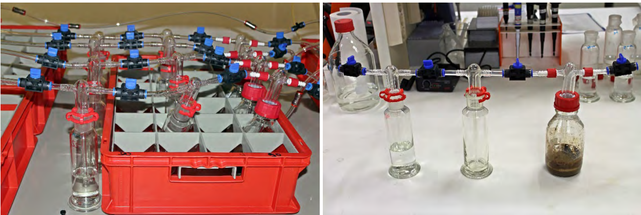
Figure 8: Pictures semi-static test apparatus used in the ring test by Institute 2
