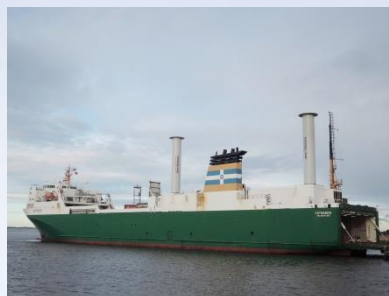
Norsepower fits twin rotors on M/V Estraden
