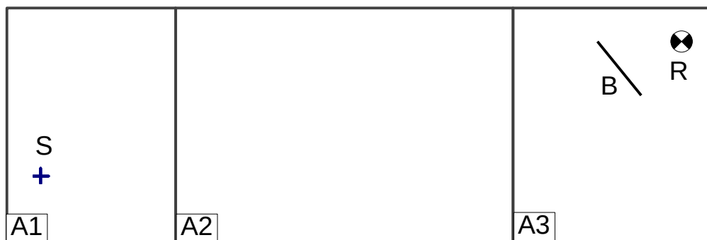
Figure 5.3.9-1: Short noise barrier on level ground with varying acoustic properties (S source, R immission point, B noise barrier, A1 area with G=0.2, A2 area with G=0.5, A3 area with G=0.9) (Source: Umweltbundesamt [9])
