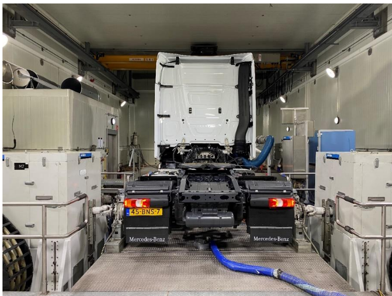
Figure 2: Mercedes-Benz in the Climatic Altitude Chamber.
