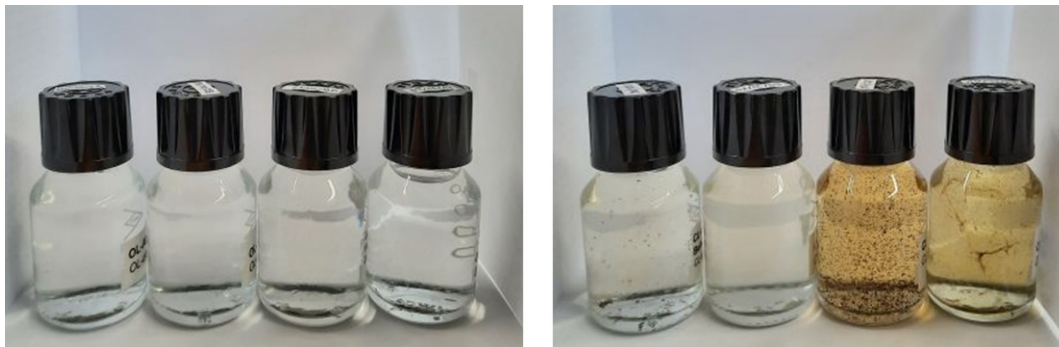
Figure 7: Samples of EGCS discharge water from the ImpEx measurement campaign: left side from OL, right side from CL mode of the hybrid systems from ships S1 to S4 16
