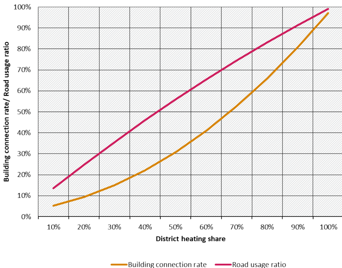
Figure 68: Average building connection rate and road usage ratio as a function of the district heating share
