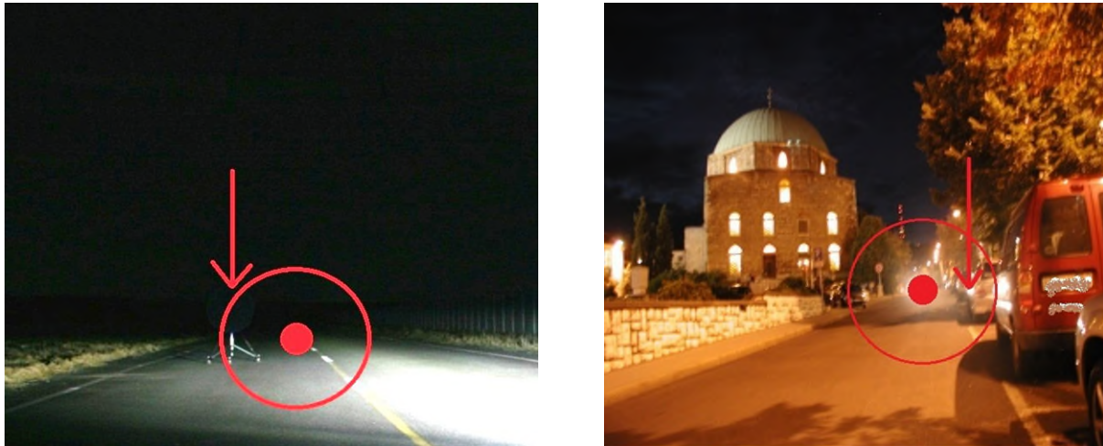
Figure 13: Comparison of the mesopic visual tasks detection and brightness assessment. Filled red circle: the central viewing field at the fixation point of the observer with a diameter of 2^\circ . Red circle: a viewing field with a diameter of 10^\circ . Left: detection of a typical mesopic object, here: an artificial grey object in a field experiment at 5^\circ in the periphery, at the red arrow. Right: mesopic brightness perception: long-term viewing of the entire street scene. The red arrow shows a possible point of appearance of an object to be detected (e.g. pedestrian) between the two parking cars
