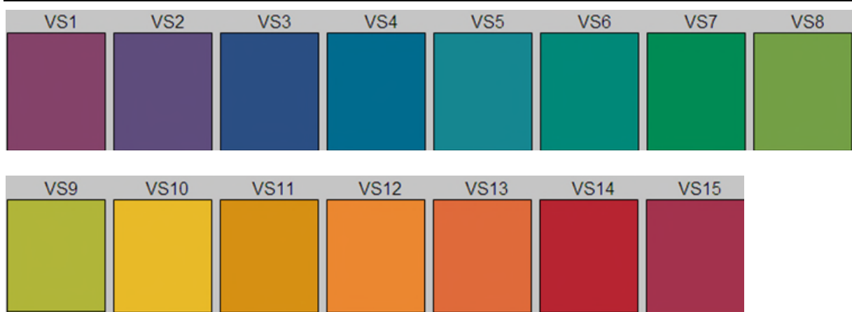
Figure 22: Test colour samples of the CQS method (NIST, USA, Version 7.1), VS1-VS15 [30]
