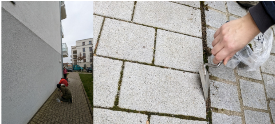
Figure 4: Sampling of joint material on pavements
