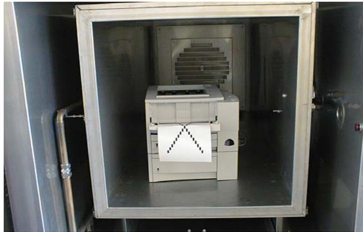
Figure K1: View of the type B 1m<sup>3</sup> emission test chamber with a printer in test
