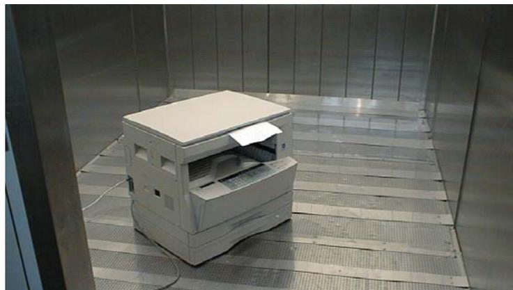
Figure K2: View of the 20m<sup>3</sup> emission test chamber with a printer in test
