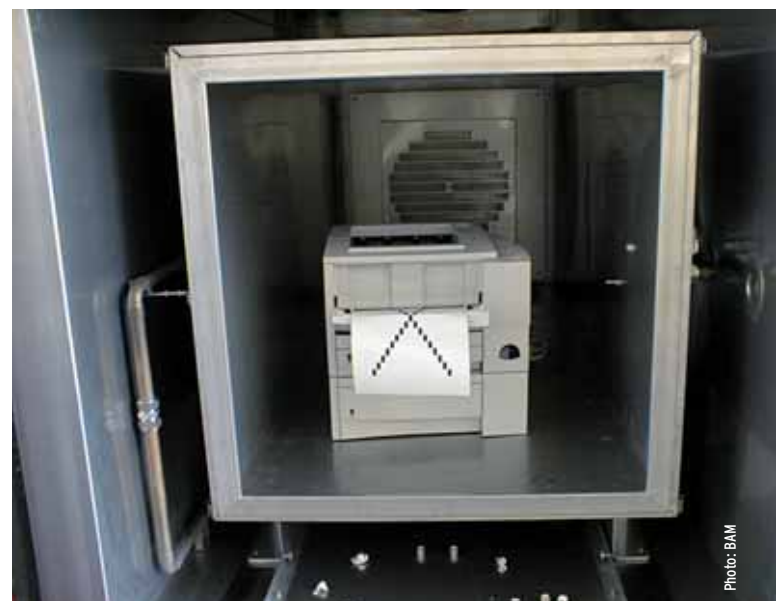
Emissions testing: Chamber with a volume of one cubic metre with a printer.
