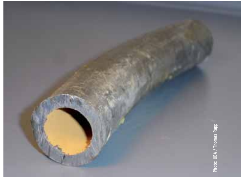
Lead pipes are a health hazard and should be completely removed without delay.
