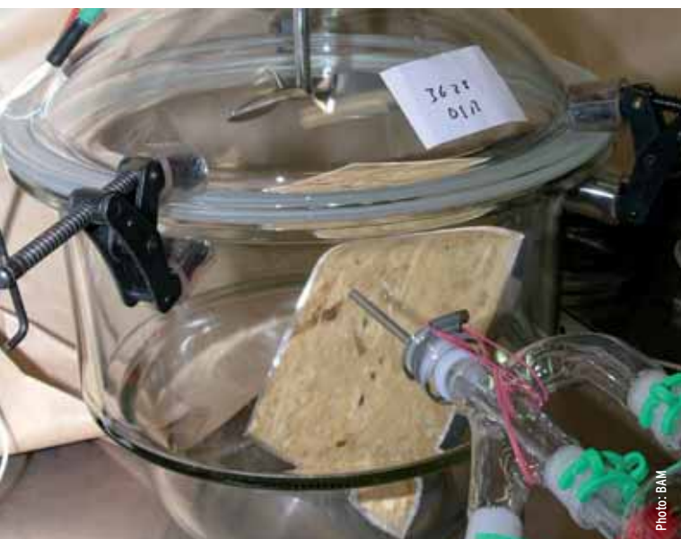
Emissions testing: Chamber with a volume of 20 litres (excicator) with a material sample consisting of a chipboard panel.
