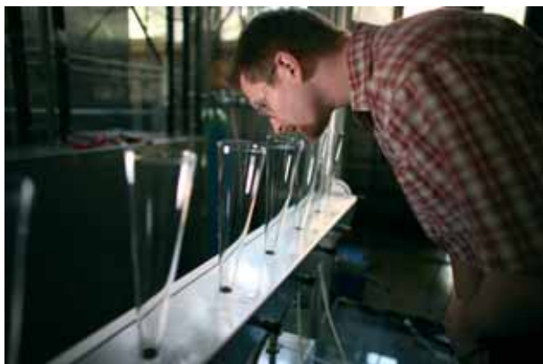
Fig. 14: Comparative samples for the testing of odour intensity. The comparative samples correspond to concentrations between 0 and 15 pi. 1 pi corresponds to the odour threshold where the comparative material is just perceptible. The more intensive the panellist perceives an odour, the greater the value pi. The scale reached to 30 in the research project. The panellists are free to extrapolate odour intensities.
