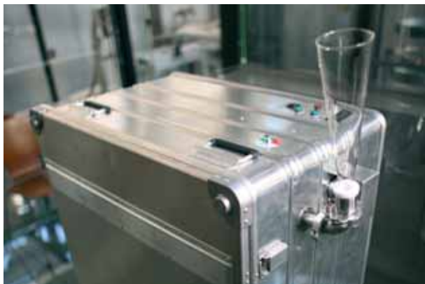
Fig. 13: Sampling and sample provision equipment Air Probe with a glass assessment funnel on the right. The panellist puts his nose over the funnel into the homogeneous flow of sample air for odour measurement.
