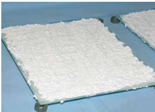
Fig. 6: Synthetic-resin premixed plaster applied to a glass plate
