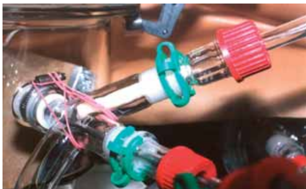
Fig. 11: A collector tube equipped with polyurethane foam (white in the picture) for adsorption of SVOC shown during sampling.
