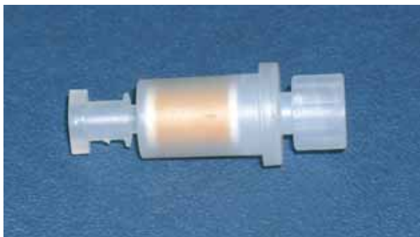
Fig. 12: Commercial collector cartridge which contains DNPH on a silica gel carrier for adsorption of aldehydes and ketones.
