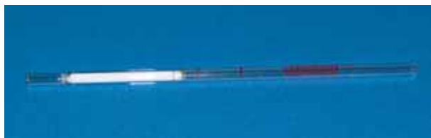
Fig. 10: Self-filled commercial Tenax TA collector tube for adsorption of VOC
