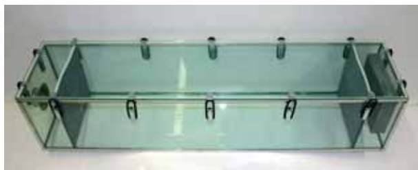
Fig. 9: View of the emission chamber CLIMPAQ with a capacity of approximately 35 litres. The room, which is intended for the material sample, is separated from the air supply and air exhaust by wire gauzes. They produce a laminar air flow encompassing the material sample.
