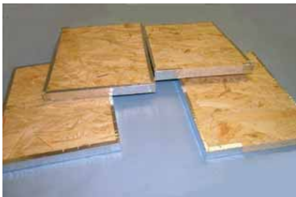
Fig. 21: OSB samples prepared for a test chamber measurement
