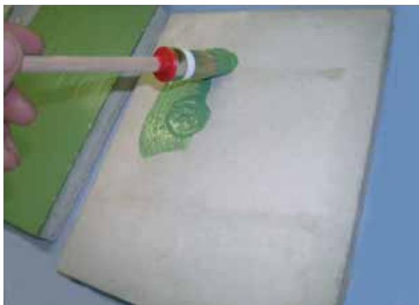
Fig. 17: Application by brush of an acrylate floor lacquer on screed in preparation for a test chamber measurement
