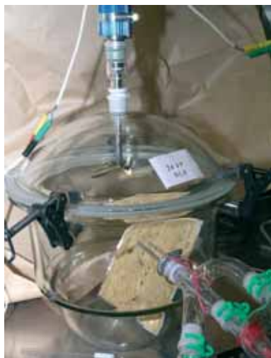
Fig. 8: Emission chamber (desiccator) with an OSB sample, capacity 20 litres
