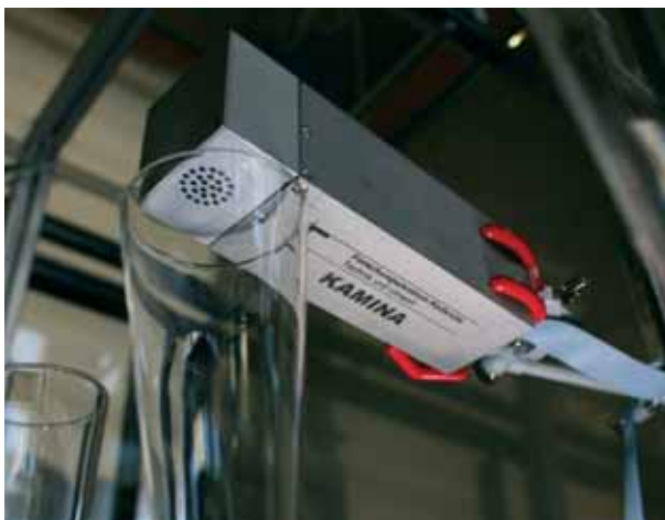
Fig. 16: The Kamina artificial nose developed by the Karlsruhe Research Centre shown above an evaluation funnel in the measuring procedure
