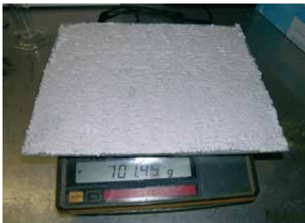
Fig. 19: Synthetic-resin premixed plaster sample on a glass plate prepared for a test chamber measurement, shown during weighing of the coated glass plate. Layer thickness recommended by the manufacturer.
