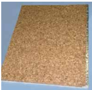
Fig. 20: Cork floor board sample prepared for a test chamber measurement
