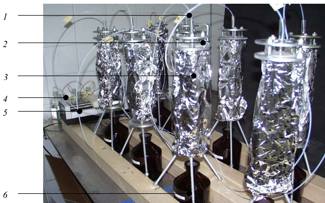
Figure 3.6: Soil columns in a soil leaching study (1: PTFE-tube; 2: glass sinter disk; 3: soil column wrapped with aluminium foil; 4: glass bottle containing artificial rain; 5: peristaltic pump; 6: leachate collecting)
