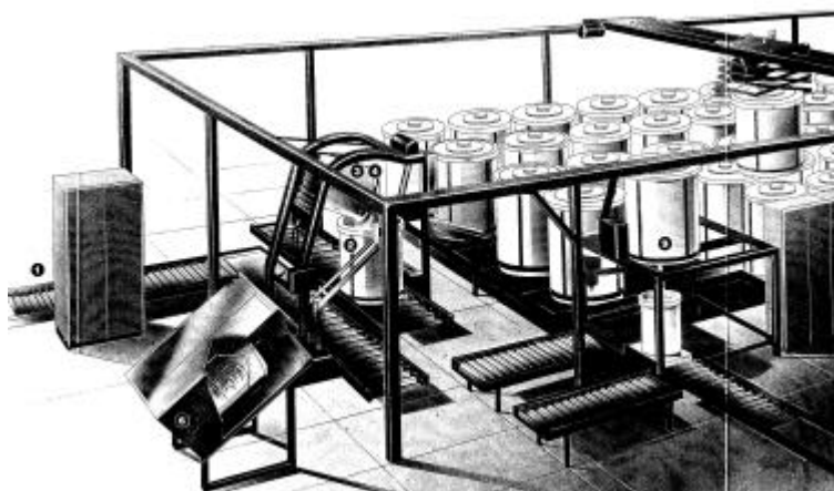
Figure 4.37: Example for printing paste recycling; the drums are emptied to certain storage tanks according to their characteristic - [Eing, 1997]
