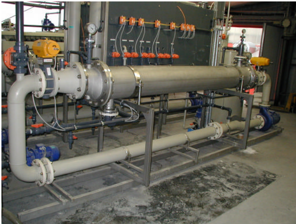
Figure 4.55: Microfiltration modul for the treatment and recycling of wastewater from a pigment paste preparation station
