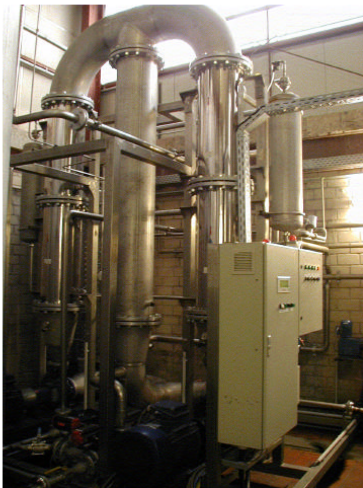
Figure 4.52: Ultrafiltration tubular moduls as part of the described plant for treatment and recycling of textile wastewater
