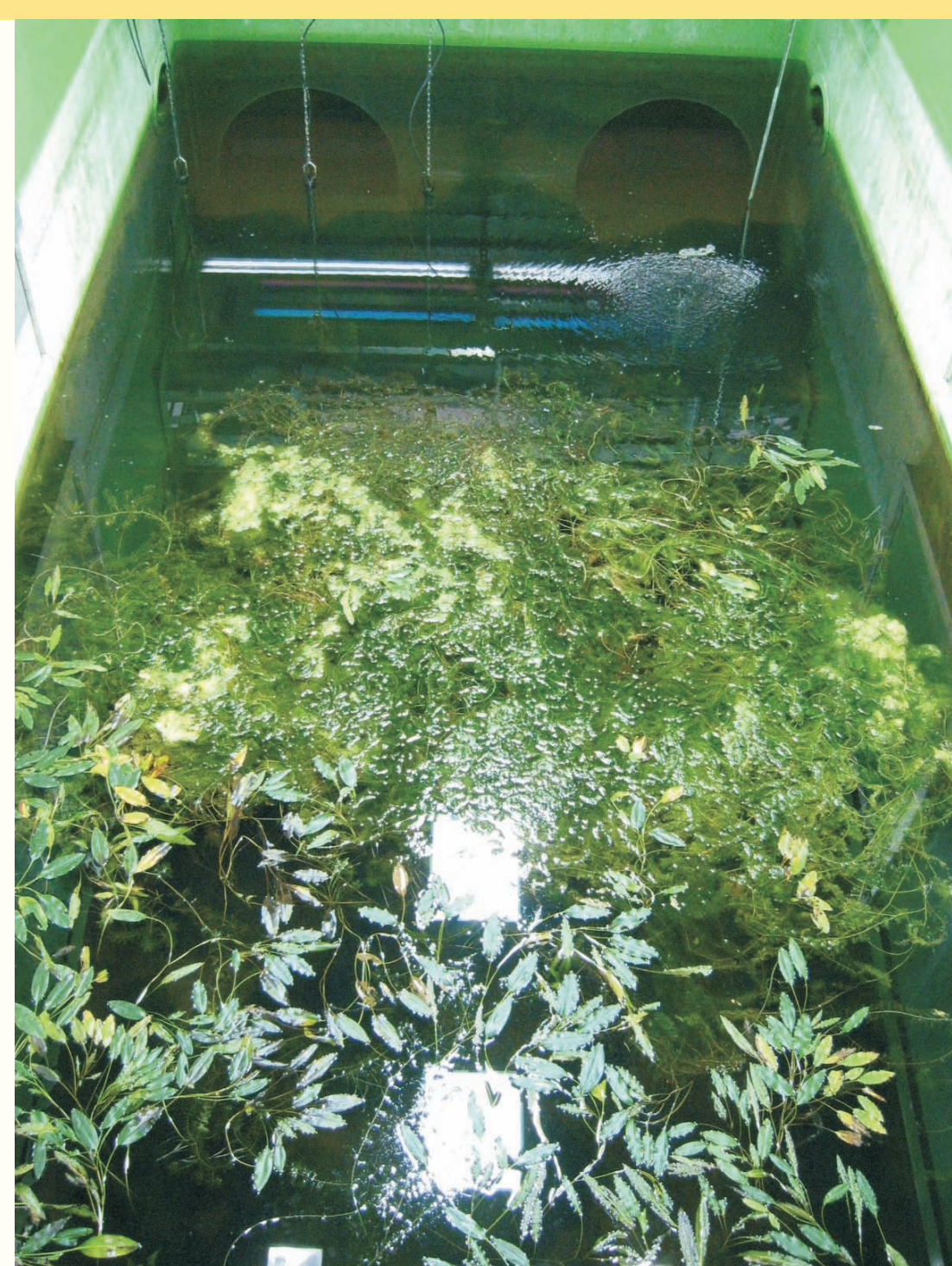
Fig. 1: Indoor pond with UV-lamps (indicated by blue reflexion), pond shown without dust protection
