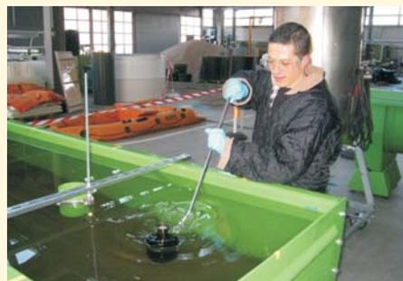
Fig. 6: Water sampling using pre-cleaned 1 L narrow-necked glass bottles
