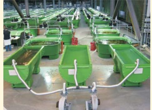
Fig. 1: Indoor pond segments of the artificial stream and pond system (FSA) of the UBA. After application of test substances, air was blown across the water surface for 30 min to ensure homogeneous distribution
