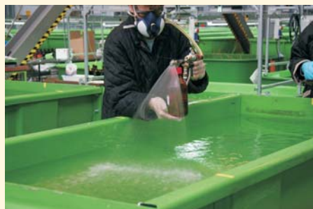
Fig. 5: Application of BDE-209 and DBDPE acetone solution in a water jet with a low pressure water injection system
