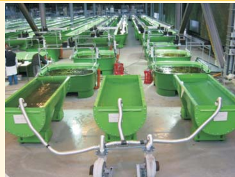
Fig. 1: Indoor pond segments of the artificial stream and pond system (FSA) of the UBA. After application of test substances, air was blown across the water surface for 30 min to ensure homogeneous distribution
