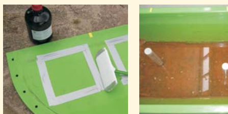
Fig. 7: Sampling of biofilms with toluene saturated cotton cloth at the end of the experiment (left) and sediment sampling using core sampler made of acrylic glass or stainless steel (right)
