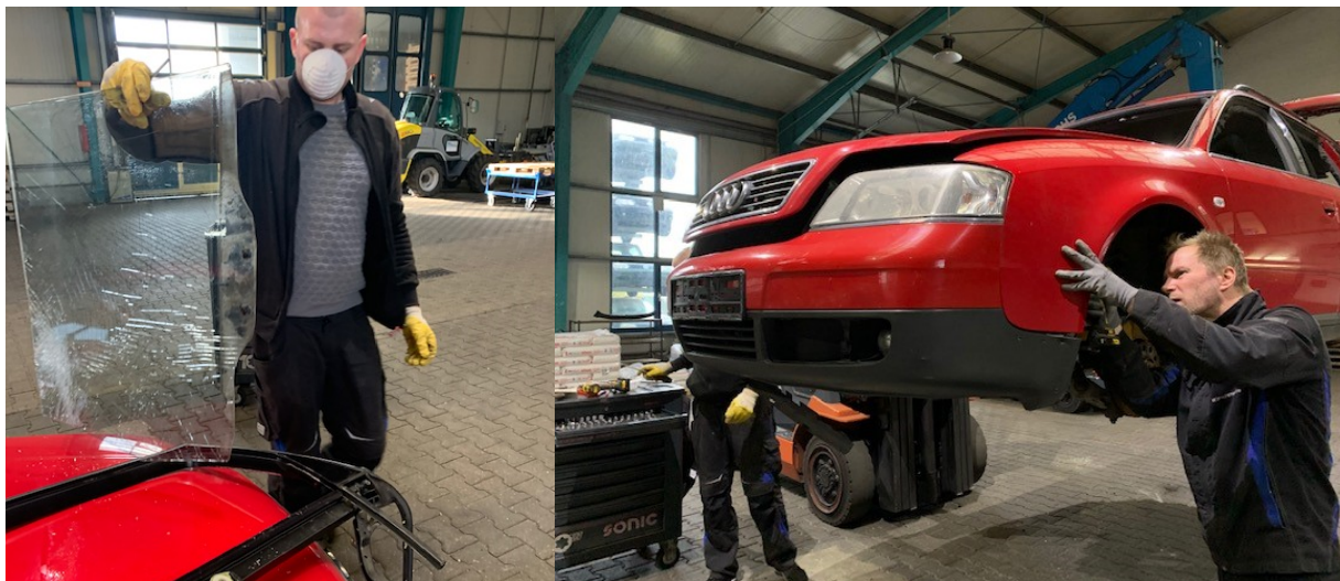
Figure 13: Dismantling of glass and plastic (bumper) from ELVs
