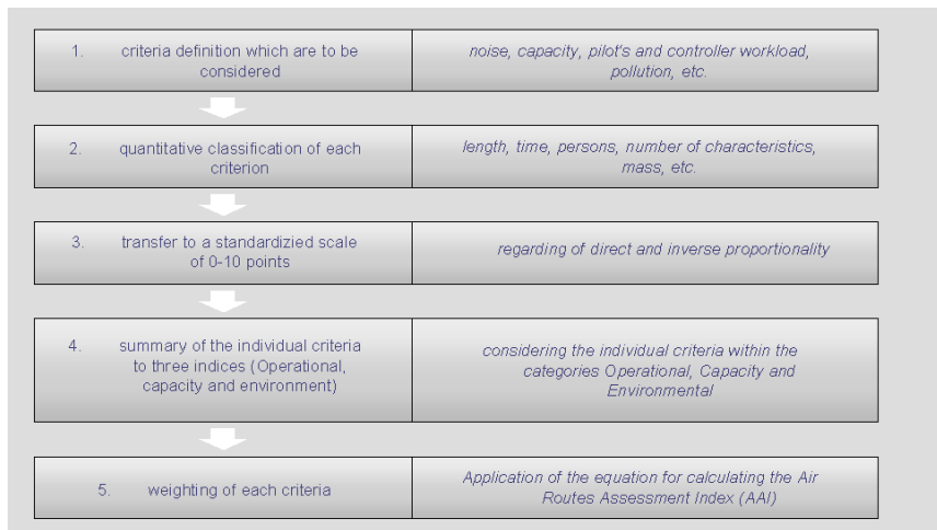
Figure 5-1: Overview of the procedure to the assessment of air routes and flight procedures
