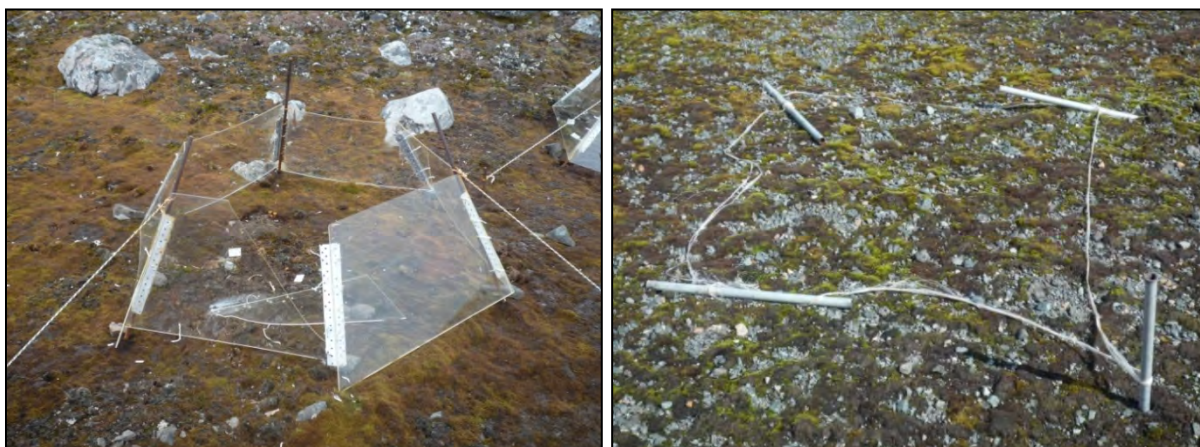
Fig. 62 a & b: Destroyed experimental equipment: (a) “open top chamber” with broken Plexiglas wall (02.01.2010), (b) fallen marker posts and frayed marking tape from a vegetation experiment (photos: A. Nordt, 12.01.2010).
