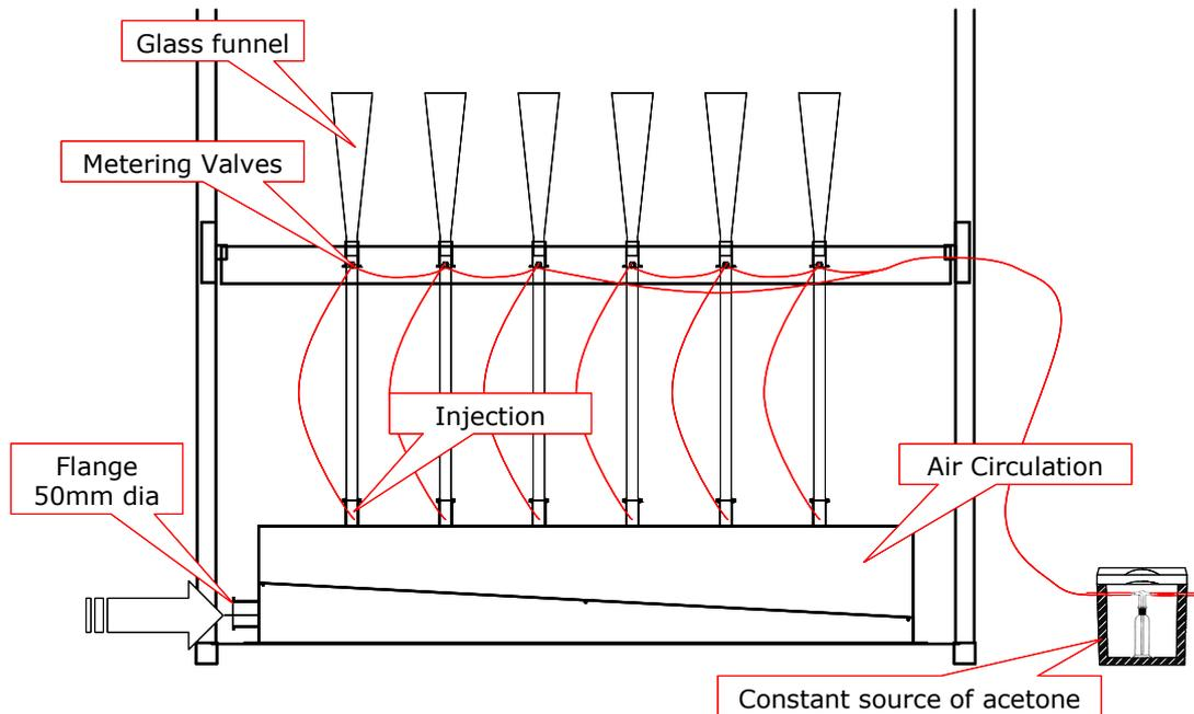
**Figure 3-4: Scheme of comparative scale**
