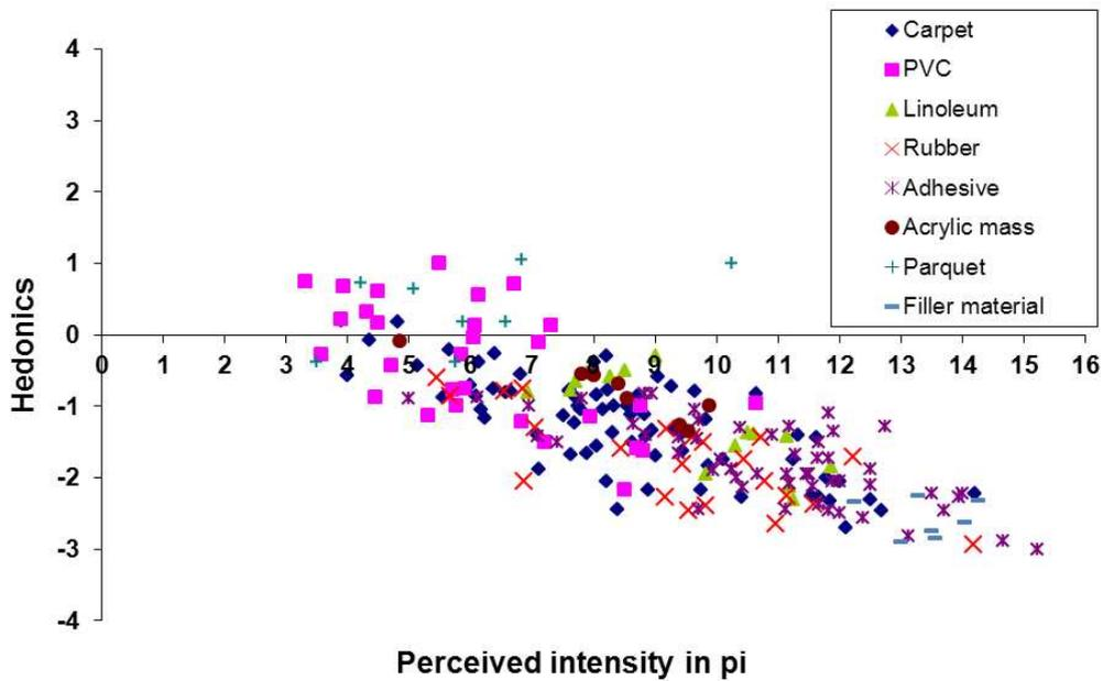
**Figure 5-7: Relationship between perceived intensity and hedonics for building products on all measurement days up to day 29**
