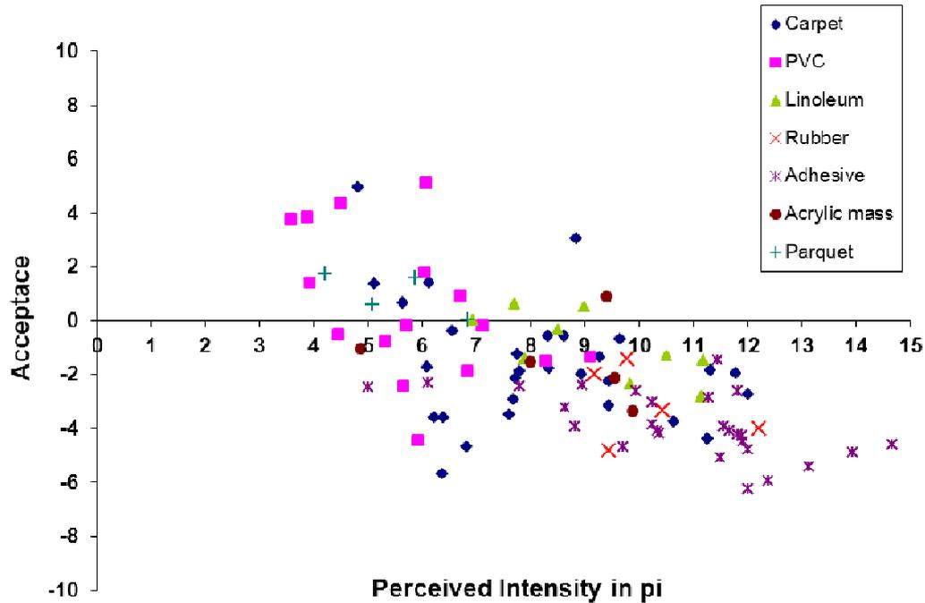
**Figure 5-5: Relationship between perceived intensity and acceptance for building products (in CLIMPAQ) on all measurement days up to day 29**
