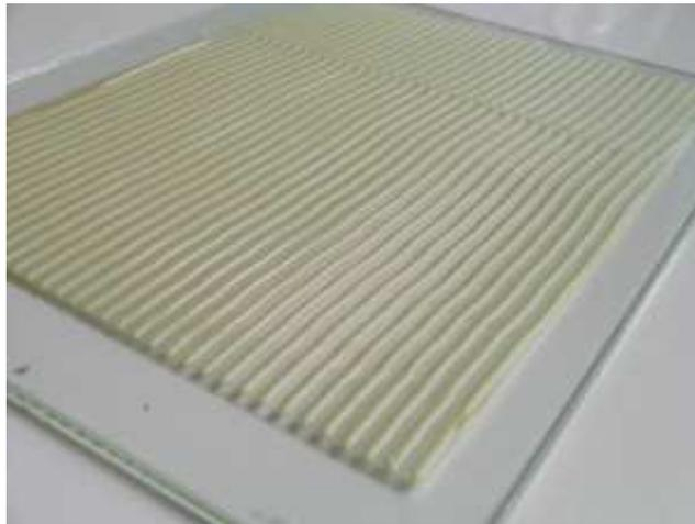
**Figure 4-15: Application of a floor covering adhesive on a glass plate**
