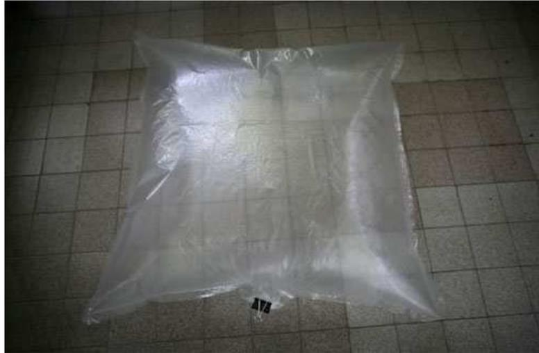
**Figure 4-11: Tedlar® container filled with sample air**
