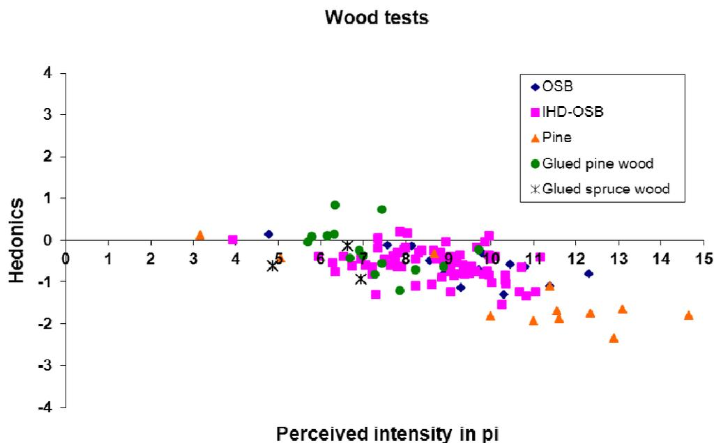
**Figure 5-10: Relationship between perceived intensity and hedonics for wood products [36] (in EXSI) over all test days up to day 29**
