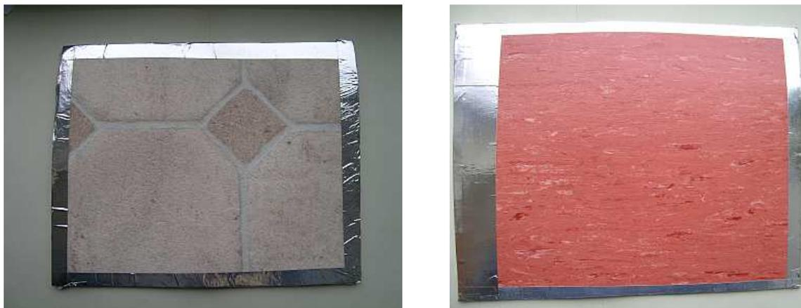
**Figure 4-14: Two PVC samples prepared for the 24-litre chambers**
