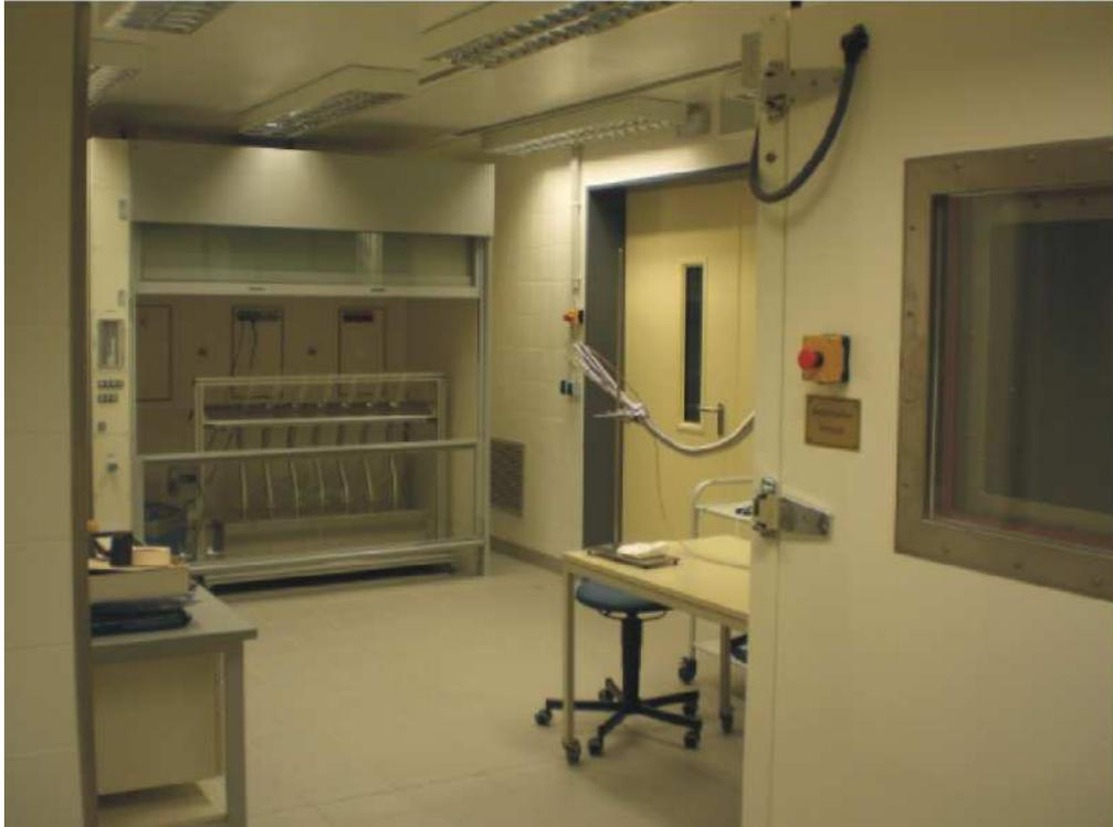
**Figure 4-28: Mobile comparative scale and 5-m<sup>3</sup> chamber with assessment funnels**
