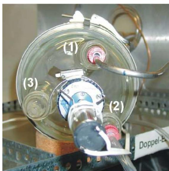
**Figure 4-26: Plane flange lid with its four openings**
