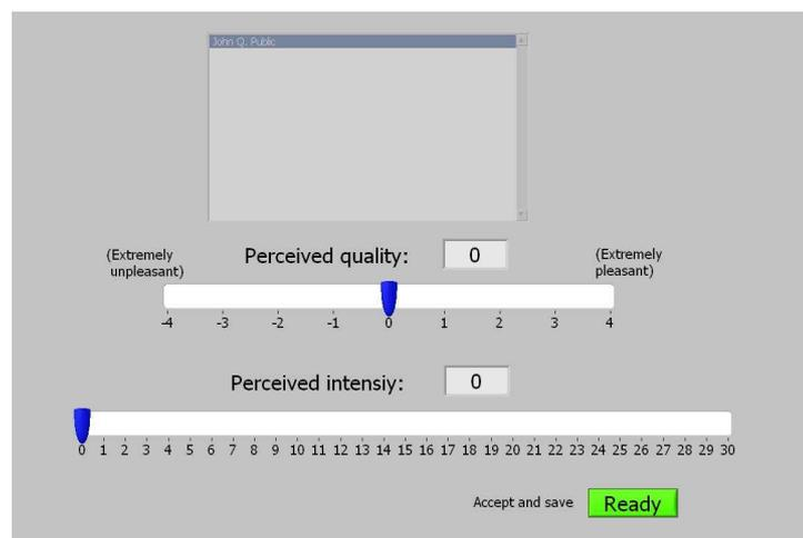
**Figure 4-16: Interface of the data acquisition software for perceived intensity evaluation by panellists using a comparative scale**
