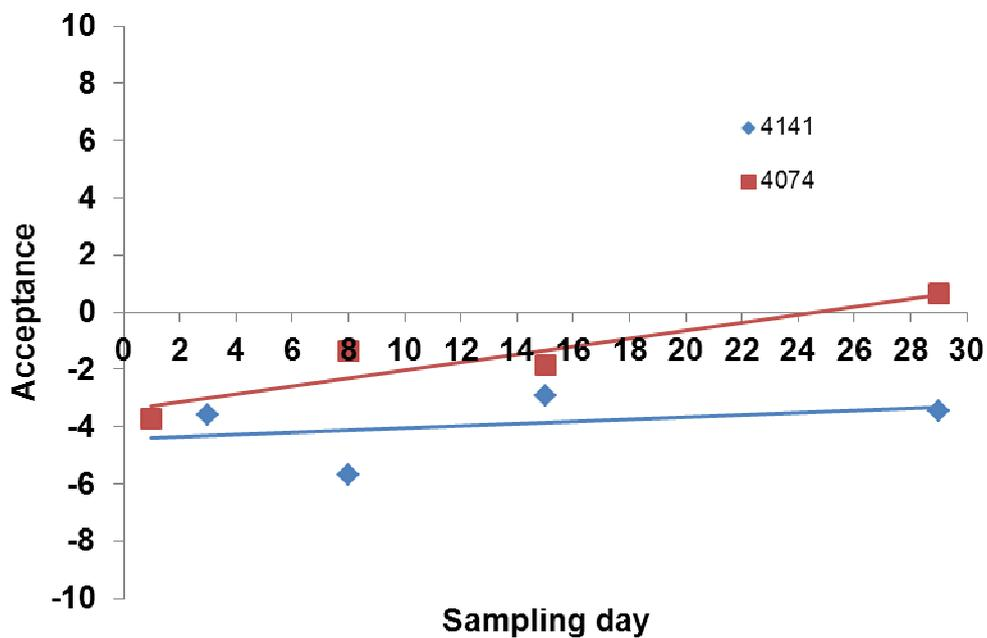
**Figure 5-3: Acceptance of wall-to-wall carpets 4141 and 4074 as a function of time**
