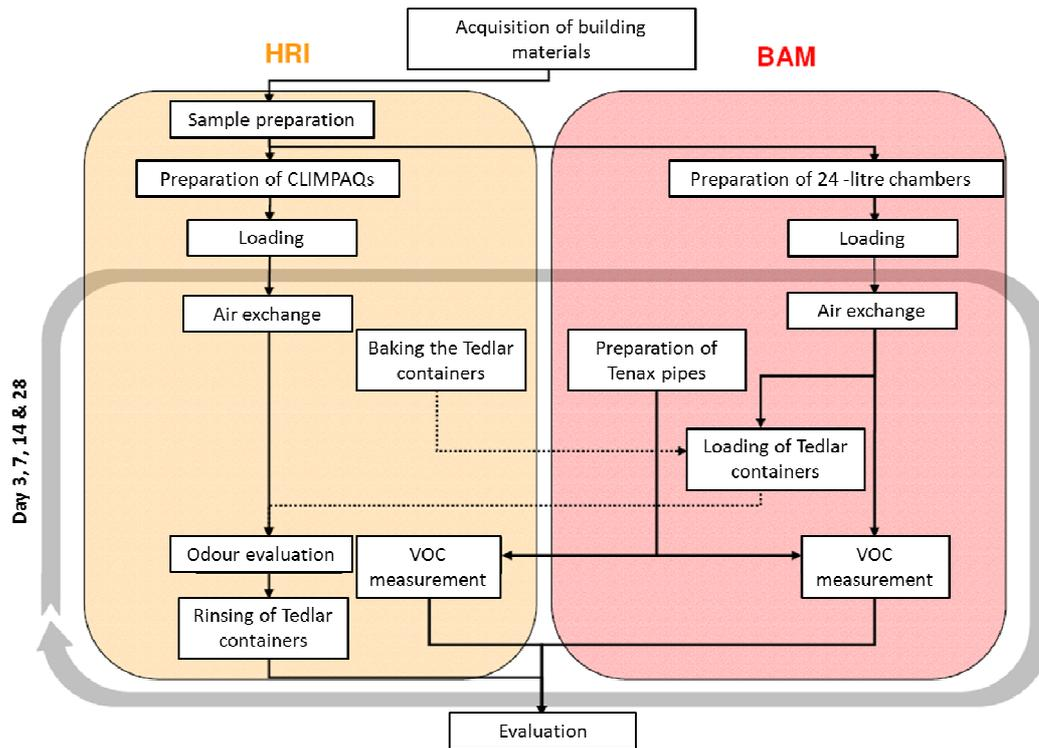
**Figure 4-1: Measurement flowchart**
