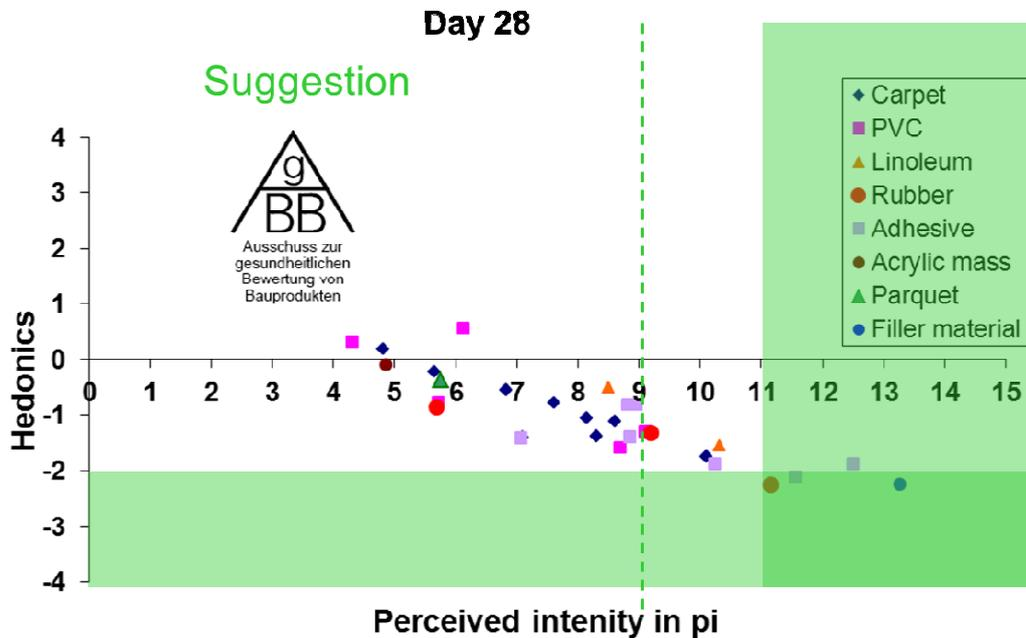
**Figure 5-54: Suggestion for the sensory-based limits for the AgBB scheme**
