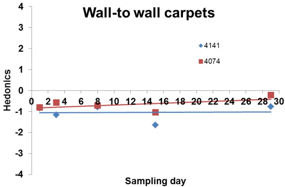
**Figure 5-2: Hedonics of wall-to-wall carpets 4141 and 4074 as a function of time**
