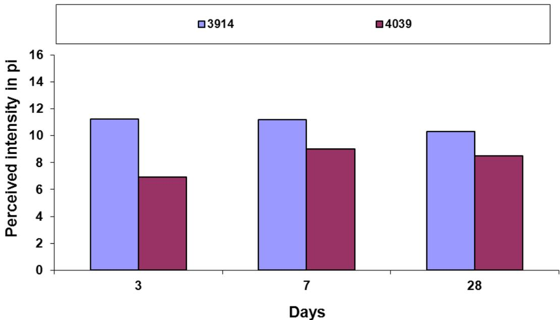
Figure 5-18: Perceived intensity of linoleum floor coverings
