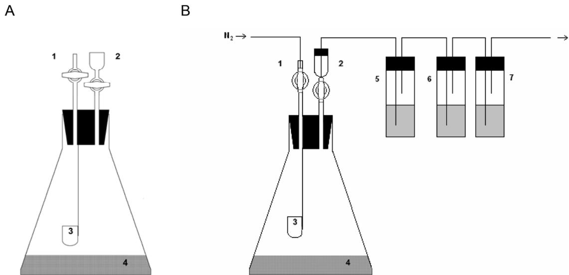
1: inlet valve, 2: outlet valve with activated charcoal filter, 3: internal  $^{14}\text{C}$ -carbon dioxide trap, 4: manure or manured soils sample, 5: external trap for  $^{14}\text{C}$ -methane with ethylene glycol (10 mL), 6: external trap with sulfuric acid (10 mL, 0.05 M), 7: external  $^{14}\text{C}$ -carbon dioxide trap with scintillation cocktail (10 mL)
