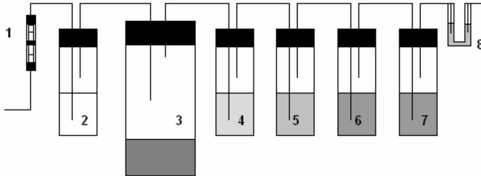
1: flow meter, 2: gas moistening flask, 3: incubation flask with the liquid manure sample, 4: ethylene glycol trap (30 mL), 5: sulfuric acid trap (30 mL, 0.05 M), 6, 7: potassium hydroxide solution traps (30 mL, 2 M), 8: bubble meter
