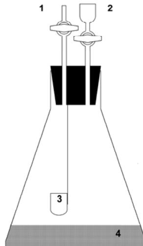
**1:** inlet valve, **2:** outlet valve with activated charcoal filter, **3:** internal  $^{14}\text{C}$ -carbon dioxide trap (8 mL of 0.1 M potassium hydroxide solution), **4:** manure or soil sample
