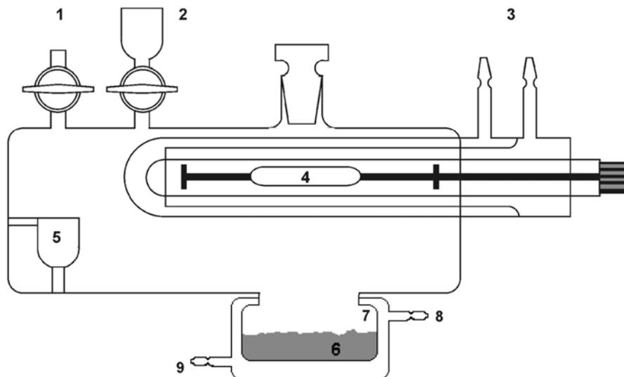
**1:** inlet valve, **2:** outlet valve with activated charcoal filter, **3:** Pyrex® water-cooling device, **4:** medium-pressure mercury lamp (cut off:  $\lambda = 290$  nm), **5:**  $^{14}\text{C}$ -carbon dioxide trap (8 mL of 0.1 M potassium hydroxide solution), **6:** soil sample, **7:** exchangeable sample container, **8,9:** water-cooling device
