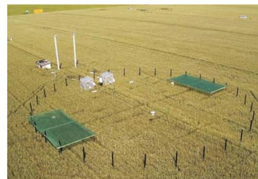
Figure 1: 20 m diameter FACE ring in a winter wheat field at Braunschweig, Germany; also shown are canopy chambers to measure CO<sub>2</sub>-/H<sub>2</sub>O-fluxes and shading devices.
