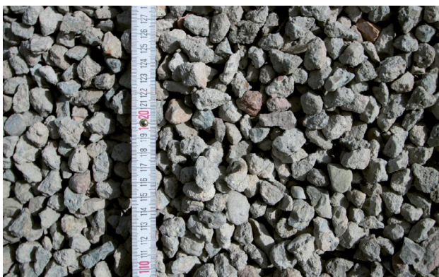
Recycled aggregate 8/16 mm from concrete
