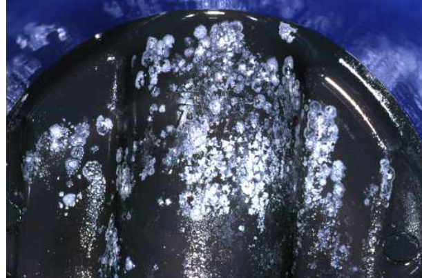
Coliforms on EPDM in a gate valve
