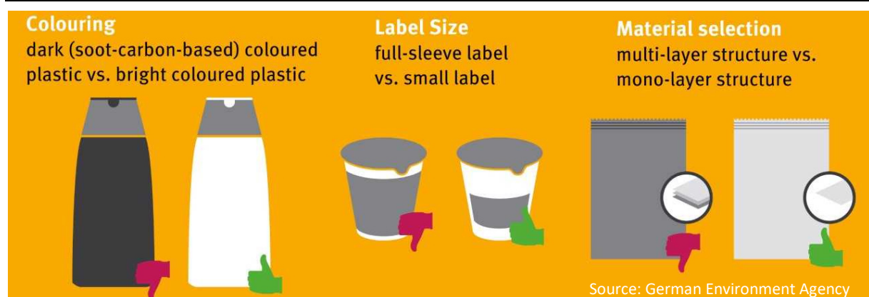
Figure 2: Comparison of the recyclability of different packaging designs
