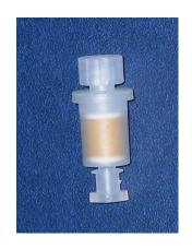
Sampling on DNPH cartridges Extraction with Acetonitrile Analysis by HPLC-UV
