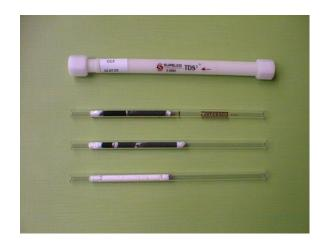
Sampling on adsorption tubes Thermal desorption (TDS) Analysis by GC-MS
