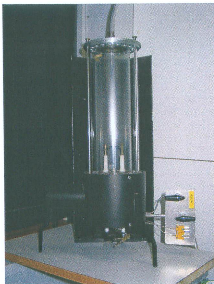
Fig. 2: Ignition tube according to DIN 51649: vertical glass tube (300 mm length, 60 mm inner diameter) and a high voltage spark ignition device 60 mm above the bottom of the tube
