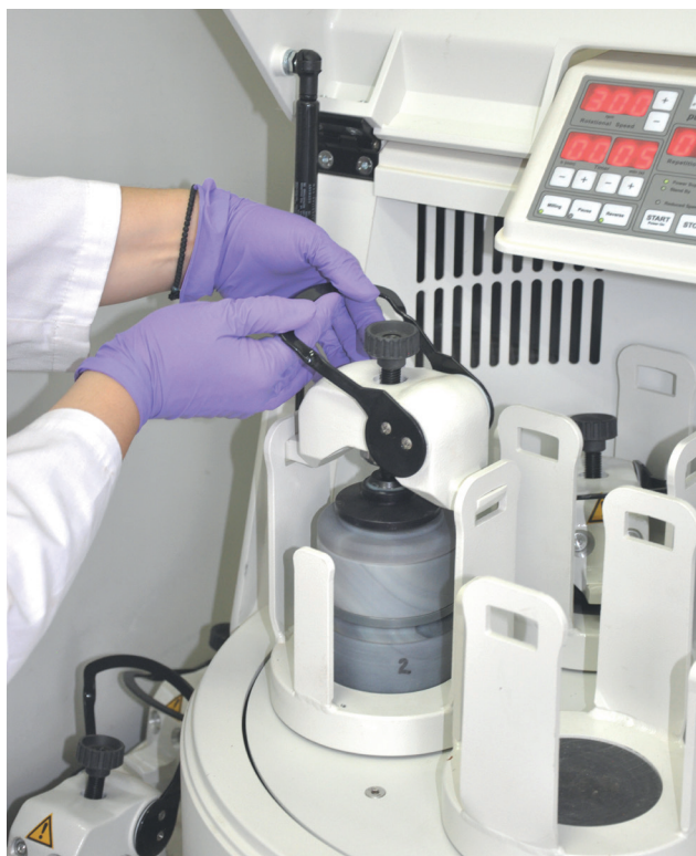
Planetary mill for fine grinding of dried samples
