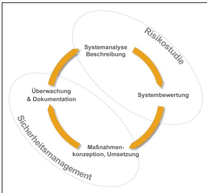
Fig. 0 1: Relationship between a risk study and (later) safety management [From top, clockwise: System analysis, description; Risk study; System assessment; Design and implementation of measures; Safety management; Monitoring and documentation]
