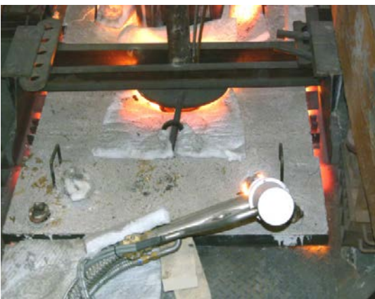
Fig. 19: Oxy-fuel diffusion burner with cooling water, used here for the feeder heating during the casting of a ship propeller in a bronze alloy (source: IfG)
