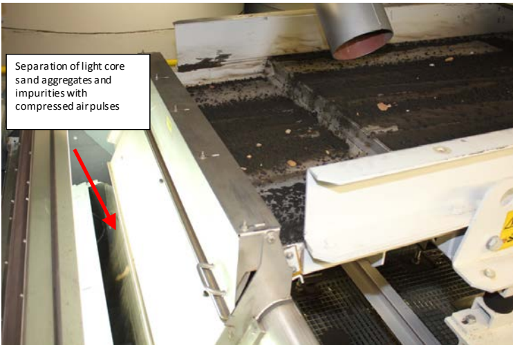
Fig. 36: Process scheme MikroSort device (source: [3])
