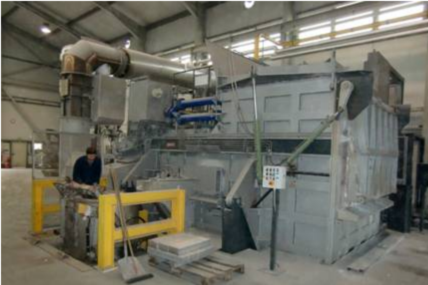
Fig. 15: The largest furnace is lowered into the ground, making it easier to clean. To drain the system, it flips into a ladle into the provided recess (source: IfG)
