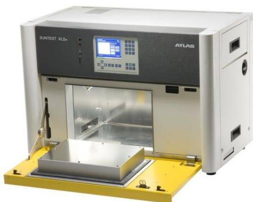
Fig. 30: SUNTEST XLS + (Atlas, Linsengericht-Altenhaßlau, Germany) without the water bath.
