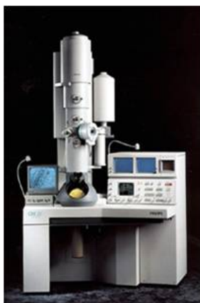
Fig. 3: Transmission electron microscope (CM 20, Philips), Ernst Ruska-Center for Microscopy and Spectroscopy, Jülich Research Center, Germany
