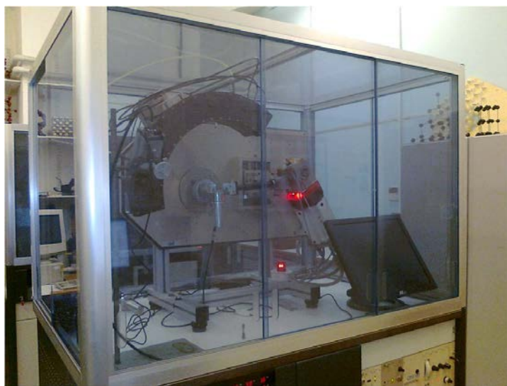
Fig. 4: X-ray powder diffractometer (FR 590 Nonius, Bruker, Billerica, USA), NHM, London, Great Britain
