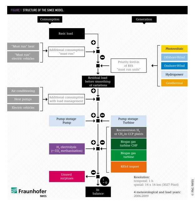
The load amount was calculated based on population, energy efficiency and "new-application assumptions" for 2050. The study cannot make predictions about altered patterns in the use of electricity technologies. We defined a "basic load curve", which covers all current types of electricity consumers, excluding the "new electricity applica-tions". This curve is based on historical load data from the European Network of Transmission System Operators for Electricity.
