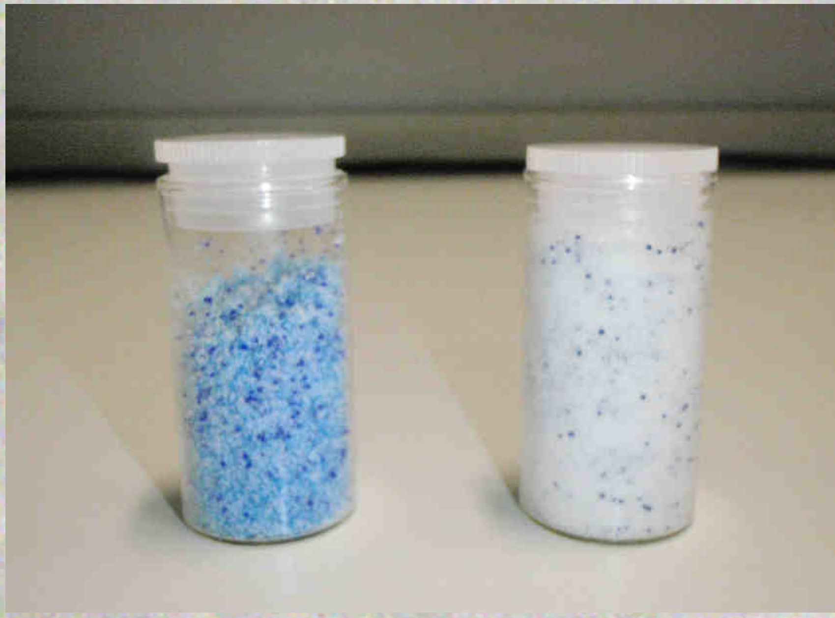
Total amount of microplastics extracted from whole tubes of face scrub.
