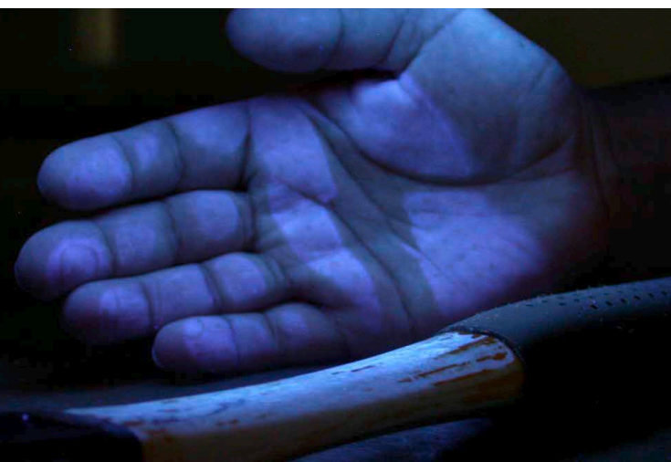
Hand (slightly creased with moisturizer) after one-time touching a rubber coated hammer shaft. The spots where PAHs were transmitted due to contact with the rubber fluoresce in UV light. Holes in the coating become visible.
