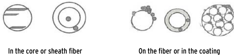
Figure 1: Ways of embedding nanomaterials in textiles (based on Bickel and Som 2011)
