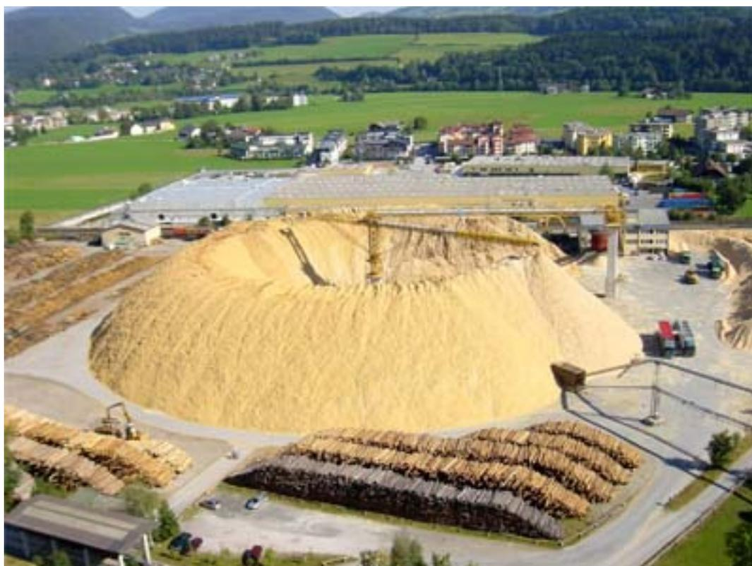
**Figure 2.5:** Example: Chip pile with concrete paving at M-real Hallein AG
