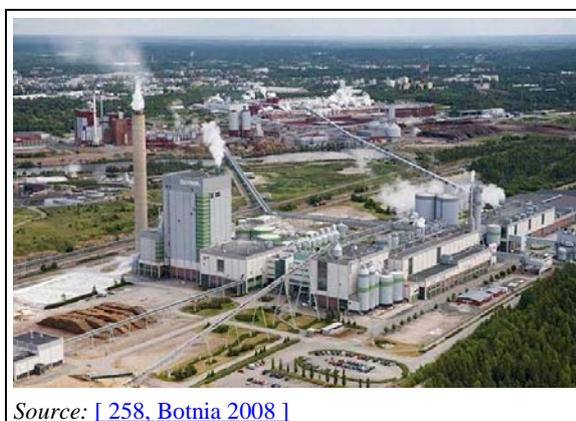
Figure 1.22: Aerial view of an integrated kraft pulp, mechanical pulp and paper site with a power plant and a waste water treatment plant
