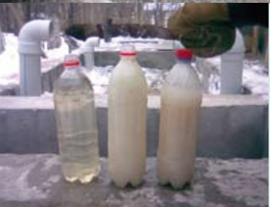
Greywater treatment in Jetygen (from right to left): influent, after pre-treatment, effluent.
