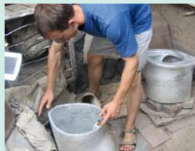
Urine diverting seat riser made from concrete.
